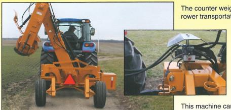
The counter weight can be positioned manually for a narrower transportation width. A hydraulically controlled counter weight is optional, for easier adjustment.
