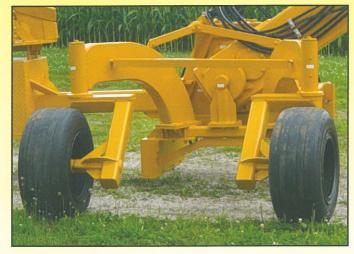
A tail wheel assembly is optional for the Ditch Angel™. This assembly helps support the weight of the machine and add stability while operating the machine.
