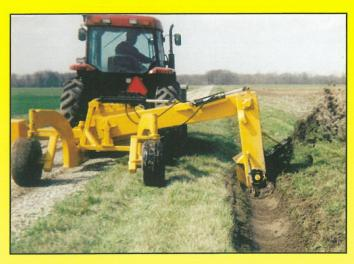
The Ditch Angel™ is a side arm ditcher. It comes equipped with a 26" ditching wheel. The ditcher operates in dry or wet conditions. It blows soil 30'-50' out the right side of the machine. A hydraulically controlled deflector is standard on all side-arm ditchers to keep material diverted away from machine and operator.
