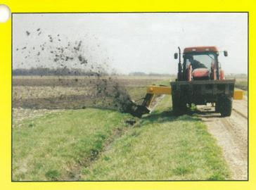
The Ditch Angel™ comes with a 26" 5 paddle impeller. Paddles are designed to be hard surfaced or carbited as they wear.
