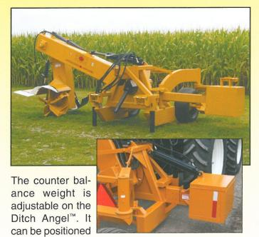
backwards (manually) to gain more clearance for transporting or storage. The counter balance can also be equipped with a hydrualic cylinder. The hydraulically controlled option allows the operator to slide the counter balance from the cab, for narrower transportation.
