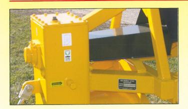
The gearbox components are easily accessible by removing the top or side cover plates. The gearbox consists of large shafts, heavy duty sprockets and bearings, double 80 roller chain; all enclosed and running in an oil bath. An external idler adjustment is easily accessible and should be used for chain tensioning. Proper chain tightening dramatically increases the life of your equipment.
