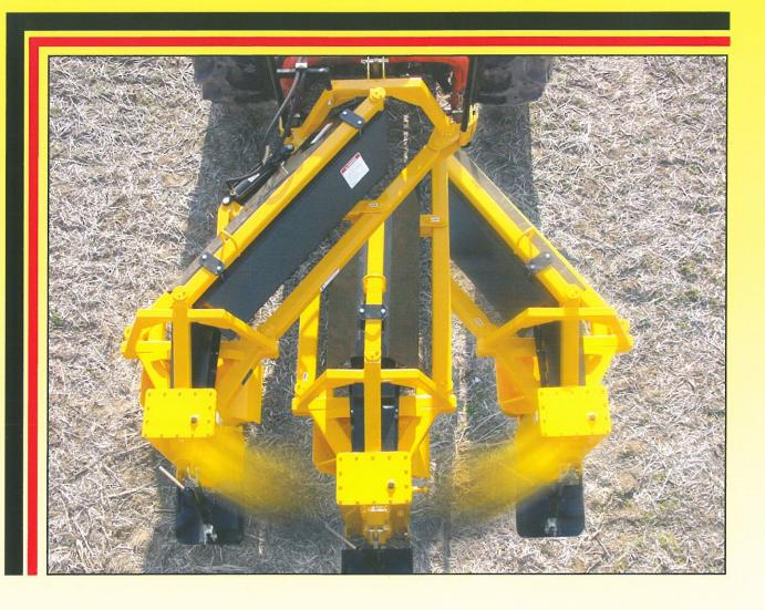
The "Swinger" is designed as an economical way to make surface drainage ditches using your own farm tractor.
