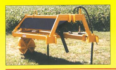
The "SWINGER" is a 3-Pt. hitch mounted machine designed to be used as an offset ditcher. It can be operated behind either tractor tire or any position in between. This ditcher accommodates any tractor with 80-140 H.P., 540 or 1000 R.P.M. P.T.O. and one hydraulic outlet.
