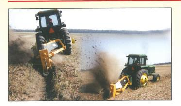
The standard 20" six paddle wheel can be replaced with a 15" five paddle wheel for smaller applications. The shoe (or dragplate) on the rear of the ditcher gives the machine stability and helps prevent gouging. The shoe is also formed to the radius of the impeller to help form the ditch in loose or wet conditions. An adjusting screw is standard on each unit for adjustment of the shoe.
