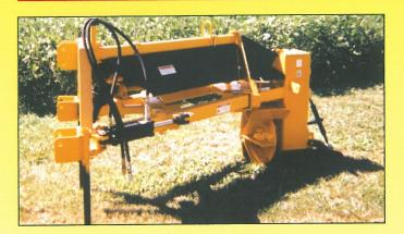
An 8" stroke cylinder hinges the machine from side to side. A 50° constant velocity (CV) joint is standard on each machine to accommodate the ditchers "SWINGING" action. It is common to cut 6-8" deep and travel about 2 1/2 M.P.H. per pass with the swinger. The power take off (P.T.O.) also contains a CV joint for smooth operation.
