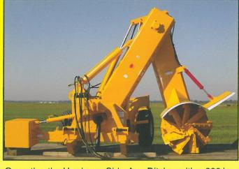
Operating the Hurricane Side-Arm Ditcher with a 200 h.p. tractor, 1 mile of ditch can be cleaned every hour, removing 10-12 inches of soil from the bottom.
