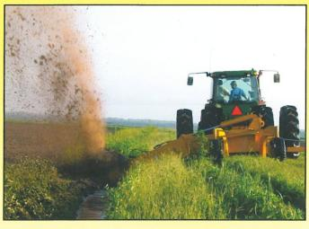
Three sets of hydraulic outlets are necessary to operate the machine. One cylinder operates each of the two arms to maintain the desired distance and depth of the ditch. The main arm contains a double 80 roller chain and the extension arm contains a triple 80 roller chain, necessary for speed reduction and machine efficiency. Each arm contains oil for chain lubrication and an idler for chain tension.
