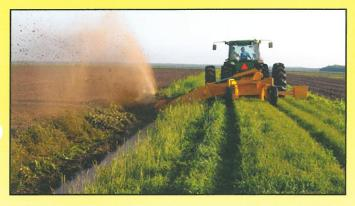
A counter balance is standard on each Hurricane Side-Arm Ditcher. This counter balance works in conjunction with the extension arm to keep the ditcher balanced in all working positions.
