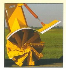
A cylinder to control the deflector is standard on each side-arm ditcher. This allows the throw of the soil to be controlled from the tractor cab instead of a manual adjustment.
